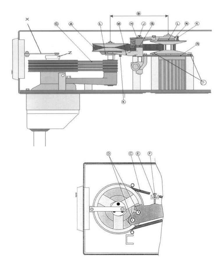
Adjustment of low and high speed microswitches.
